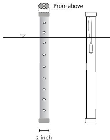
The panel above shows the installation of the diver using a 2-inch PVC pipe drilled down from the peat surface. The pipe acts like a well with as many holes as possible to allow the well to fill with water. The well should be driven into the soil at the lowest groundwater table depth level.
