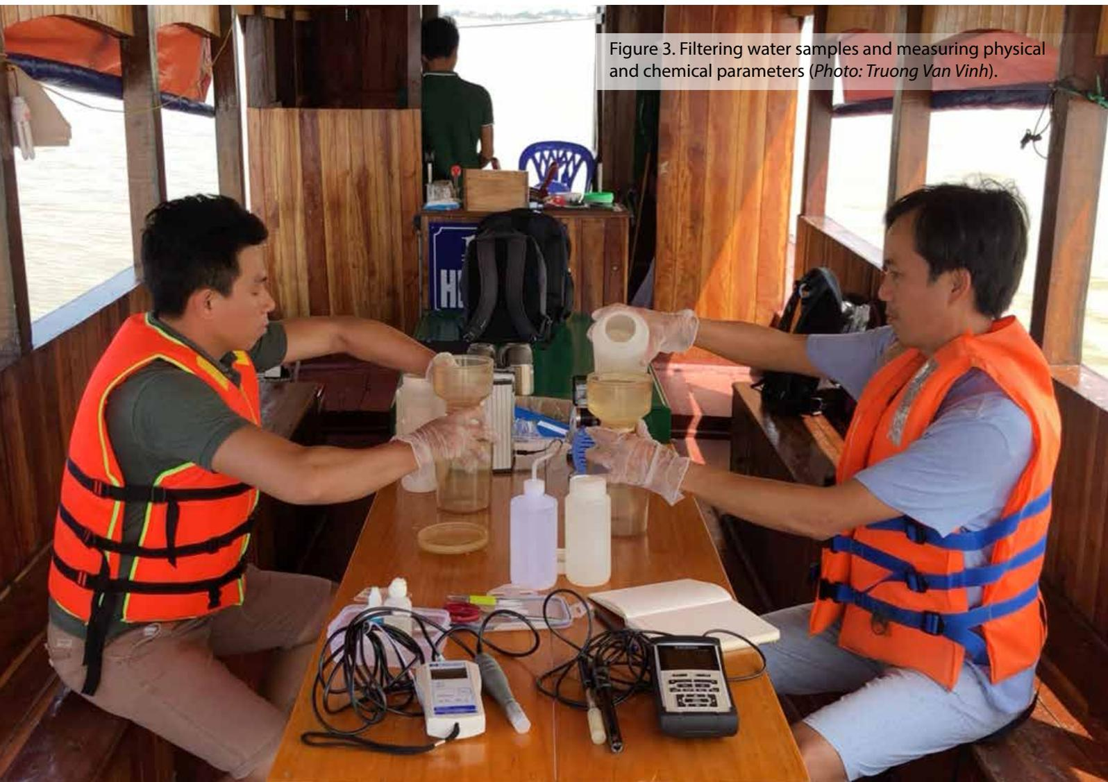
Figure 3. Filtering water samples and measuring physical and chemical parameters (Photo: Trương Văn Vinh).
