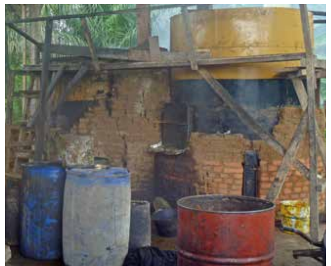
Picture 6. In-built metallic drums for CPO clarification
