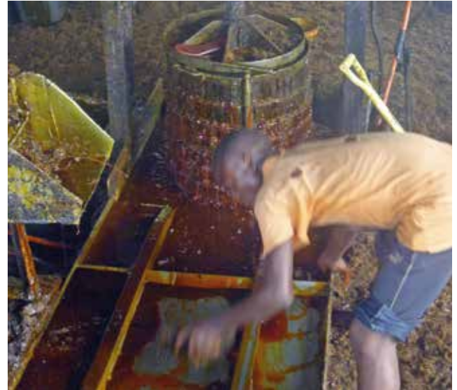
Picture 11. Crushed material pressed to extract RPO using hydraulic press
