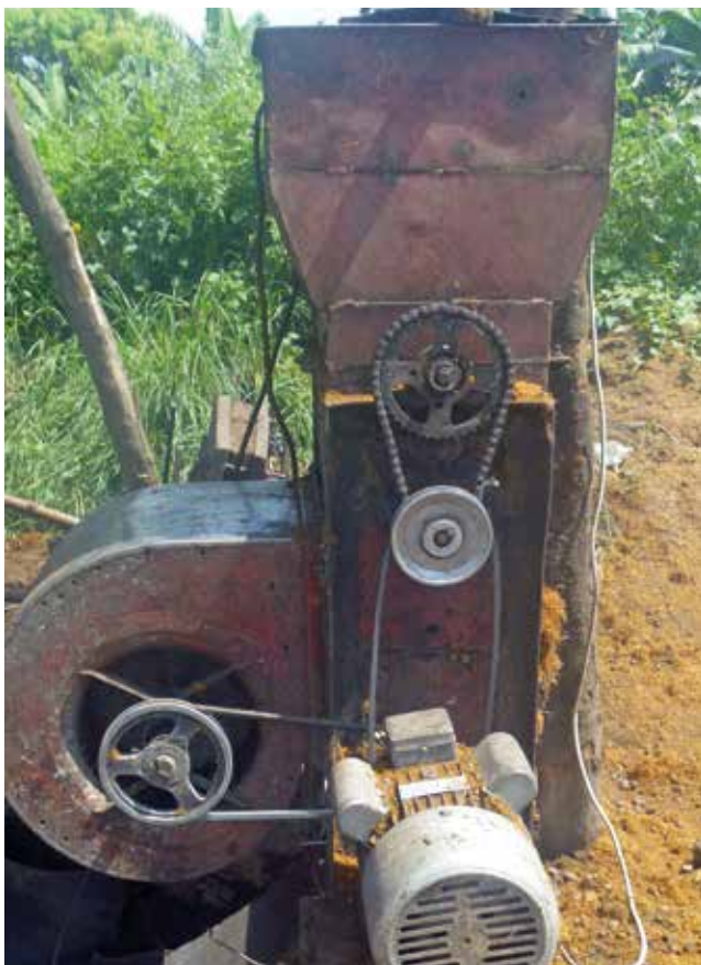
Picture 14. Fiber-kernel separator
