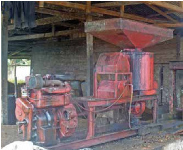
Picture 3. Combined motorized hydraulic machine and press system
