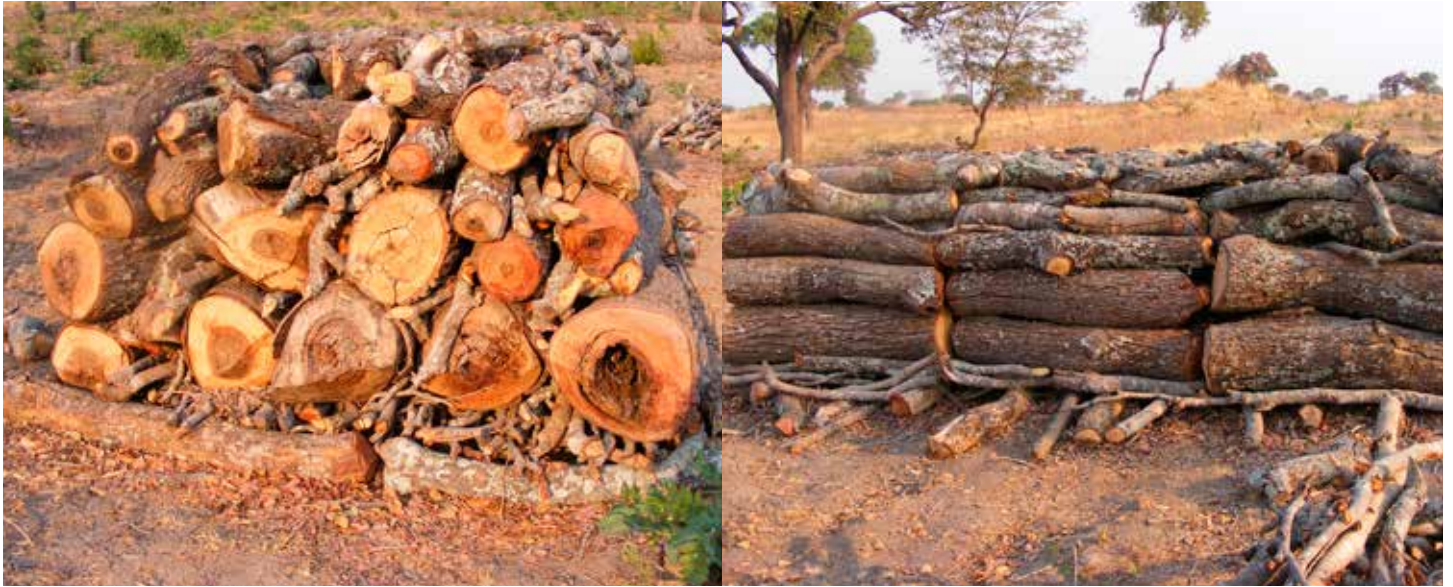
Kiln under construction on land cleared for cultivation in Nyimba district, Zambia
