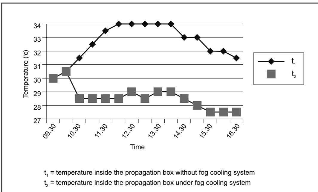
transpiration of the cutting leading to cutting dehydration. Successful vegetative propagation of the dipterocarps appears to require a condition in which the cuttings receive enough light but the temperature must be kept below 30°C.
