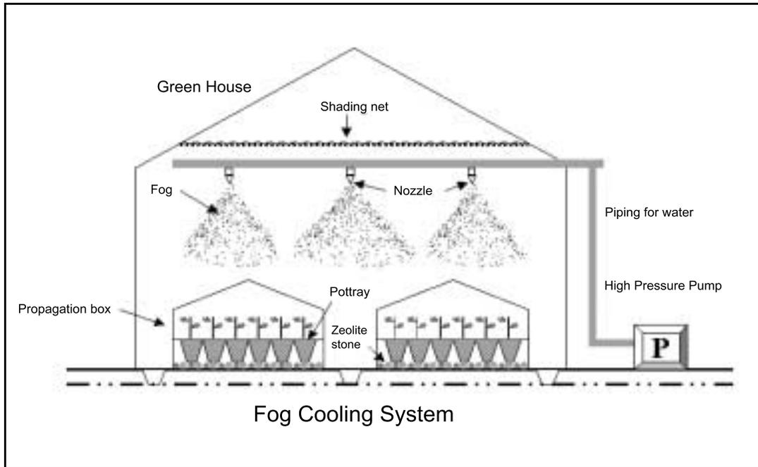
**Figure 2.** Temperature control by fog cooling system
